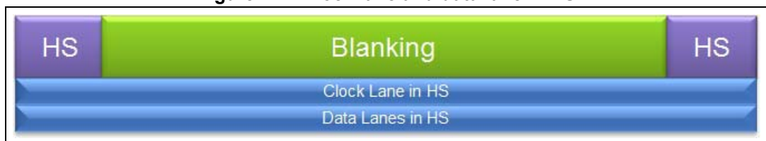
Figure 277. Clock lane and data lane in HS
