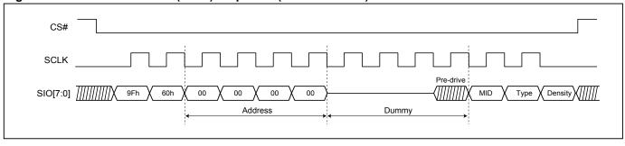
Figure 13. Read Identification (RDID) Sequence (DTR-OPI Mode)
