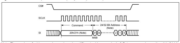
Note: The number of address cycles are based on different address mode. In 3-Byte command operation, it is 24-bit. In 4-Byte command operation, it is 32-bit.
