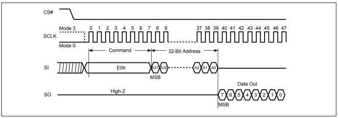
Figure 93. Read DPB Register (RDDPB) Sequence (STR-OPI Mode)
