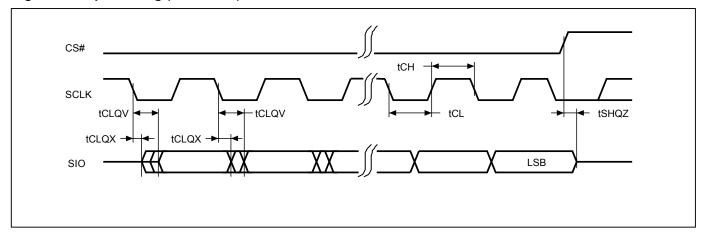
Figure 4. Output Timing (DTR mode)
