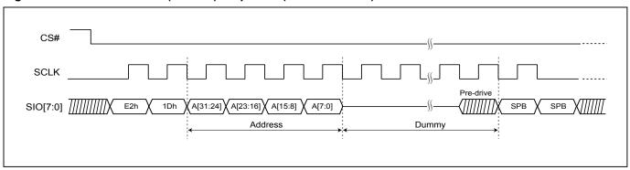
Figure 85. Read SPB Status (RDSPB) Sequence (DTR-OPI Mode)
