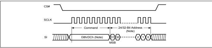
Note: The number of address cycles are based on different address mode. In 3-Byte command operation, it is 24-bit. In 4-Byte command operation, it is 32-bit.
