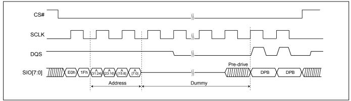
Figure 94. Write DPB Register (WRDPB) Sequence
