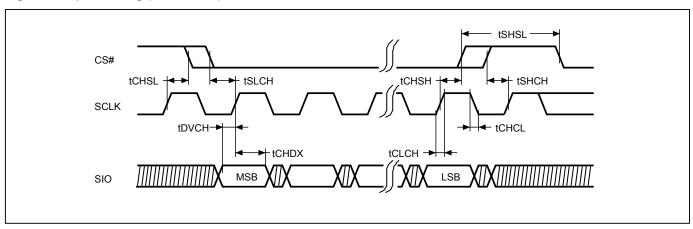
Figure 2. Input Timing (DTR mode)
