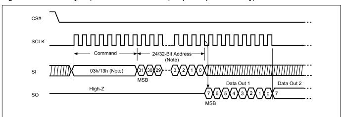
Figure 40. Read Data Bytes (READ/READ3B/READ4B) Sequence (SPI Mode only)
