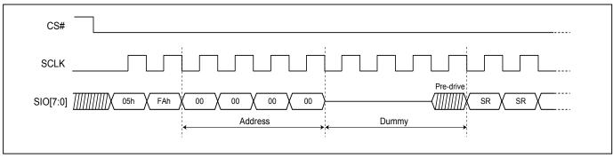
Figure 16. Read Status Register (RDSR) Sequence (DTR-OPI Mode)
