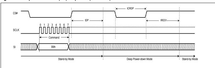
Figure 73. Deep Power-down (DP) Sequence (SPI Mode)
