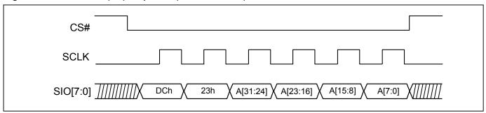
Figure 66. Block Erase (BE) Sequence (DTR-OPI Mode)
