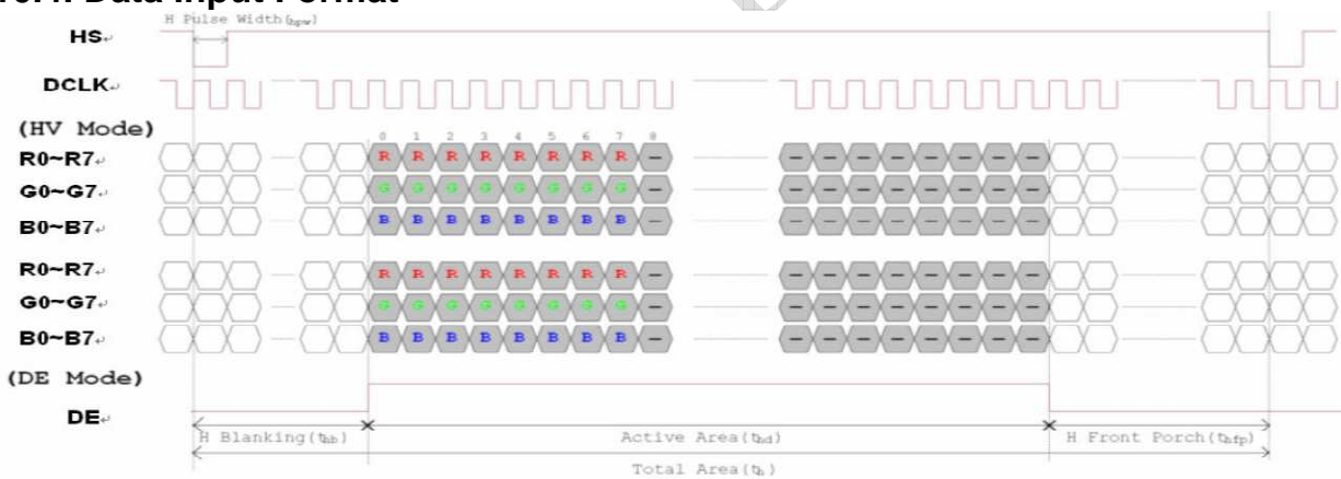
Figure 3. 1 Horizontal input timing diagram.
