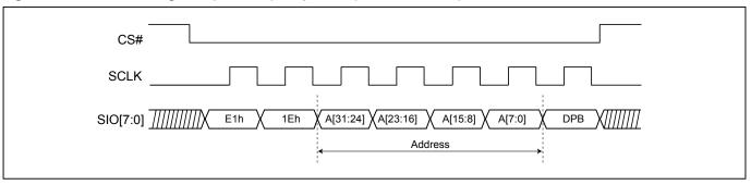
Figure 97. Write DPB Register (WRDPB) Sequence (DTR-OPI Mode)
