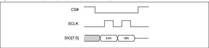
Figure 88. SPB Erase (ESSPB) Sequence (DTR-OPI Mode)
