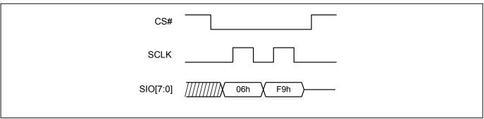
Figure 7. Write Enable (WREN) Sequence (DTR-OPI Mode)
