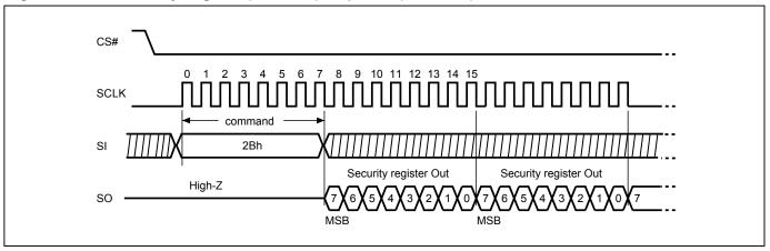
Figure 35. Read Security Register (RDSCUR) Sequence (STR-OPI Mode)
