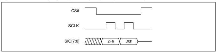
Figure 39. Write Security Register (WRSCUR) Sequence (DTR-OPI Mode)
