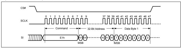
Figure 95. Write DPB Register (WRDPB) Sequence (STR-OPI Mode)
