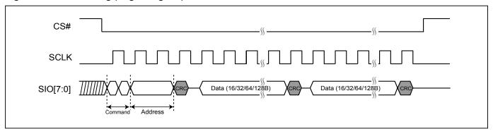
Figure 121. CRC Timing (Write Register - example for 1byte data)
