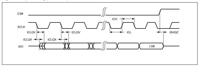
Figure 4. Output Timing (DTR mode)
