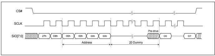
Figure 100. Read Password Register (RDPASS) Sequence (DTR-OPI Mode)
