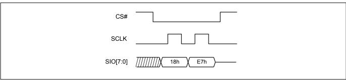
Figure 60. Erase Fast Boot Register (ESFBR) Sequence (DTR-OPI Mode)
