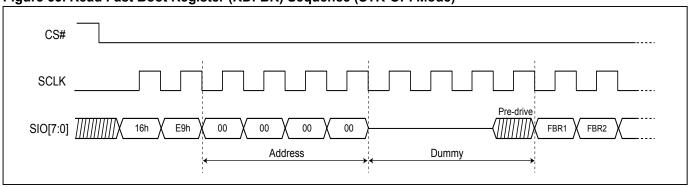
Figure 54. Read Fast Boot Register (RDFBR) Sequence (DTR-OPI Mode)
