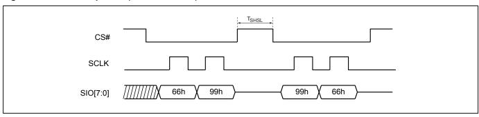
Figure 113. Reset Sequence (DTR-OPI mode)
