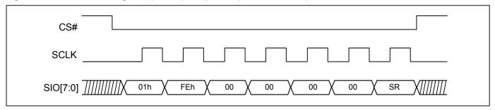
Figure 24. Write Status Register (WRSR) Sequence (DTR-OPI Mode)
