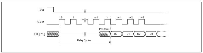
Note: If FBSD = 11, delay cycles is 21 and n is 20. If FBSD = 10, delay cycles is 17 and n is 16. If FBSD = 01, delay cycles is 15 and n is 14. If FBSD = 00, delay cycles is 11 and n is 10.
