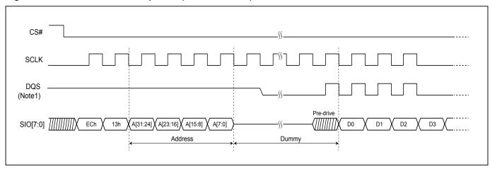
Note1: DQS is enabled only when DOS (DQS on STR mode) bit is set. Otherwise, it keeps Hi-Z.
