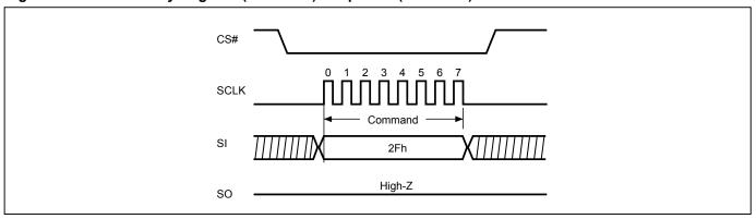
Figure 38. Write Security Register (WRSCUR) Sequence (STR-OPI Mode)
