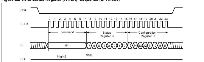
Figure 22. Write Status Register (WRSR) Sequence (SPI Mode)
