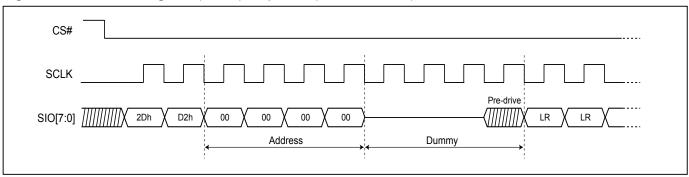
Figure 79. Read Lock Register (RDLR) Sequence (DTR-OPI Mode)
