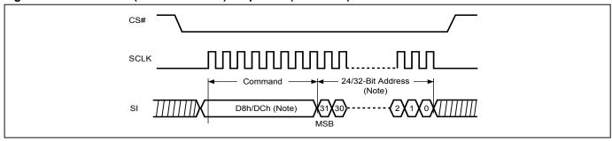
Note: The number of address cycles are based on different address mode. In 3-Byte command operation, it is 24-bit. In 4-Byte command operation, it is 32-bit.
