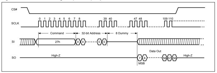
Figure 99. Read Password Register (RDPASS) Sequence (STR-OPI Mode)
