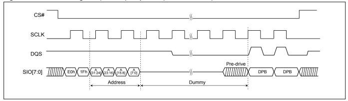
Figure 94. Write DPB Register (WRDPB) Sequence
