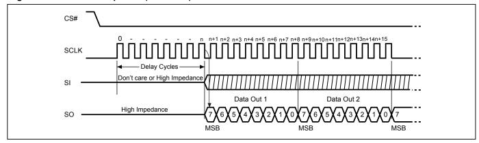
Note: The delay cycle is always 13 in SPI mode.
