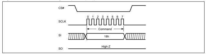
Figure 59. Erase Fast Boot Register (ESFBR) Sequence (STR-OPI Mode)
