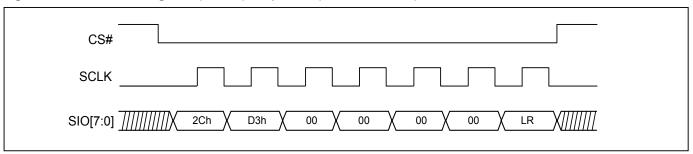
Figure 82. Write Lock Register (WRLR) Sequence (DTR-OPI Mode)
