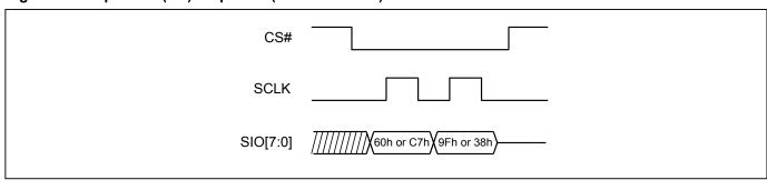
Figure 69. Chip Erase (CE) Sequence (DTR-OPI Mode)
