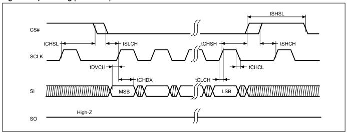
Figure 2. Input Timing (DTR mode)
