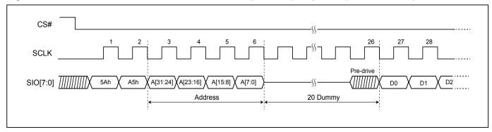
Figure 116. Read Serial Flash Discoverable Parameter (RDSFDP) Sequence (DTR-OPI Mode)
