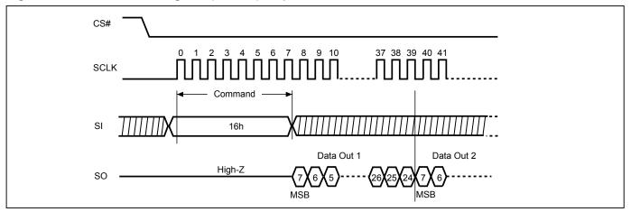
Figure 53. Read Fast Boot Register (RDFBR) Sequence (STR-OPI Mode)
