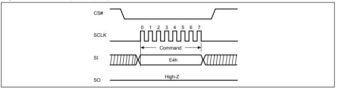
Figure 87. SPB Erase (ESSPB) Sequence (STR-OPI Mode)
