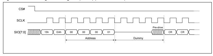
Figure 21. Read Configuration Register (RDCR) (DTR-OPI Mode)
