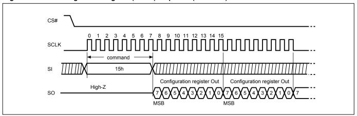
Figure 20. Read Configuration Register (RDCR) (STR-OPI Mode)
