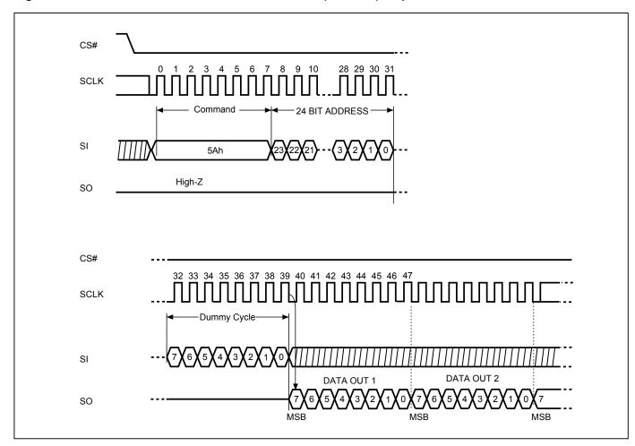
Figure 115. Read Serial Flash Discoverable Parameter (RDSFDP) Sequence (STR-OPI Mode)
