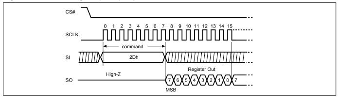
Figure 78. Read Lock Register (RDLR) Sequence (STR-OPI Mode)
