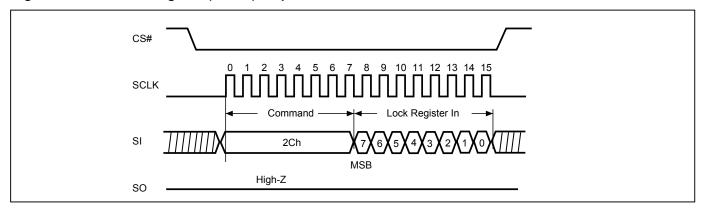
Figure 81. Write Lock Register (WRLR) Sequence (STR-OPI Mode)
