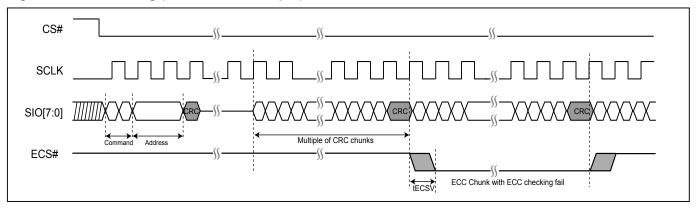
Figure 119. CRC Timing (With CRC# output)
