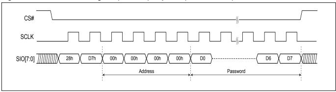
Figure 103. Write Password Register (WRPASS) Sequence (DTR-OPI Mode)
