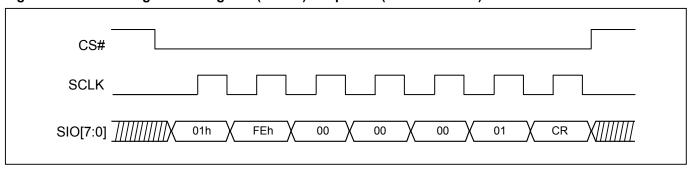
Figure 26. Write Configuration Register (WRCR) Sequence (DTR-OPI Mode)
