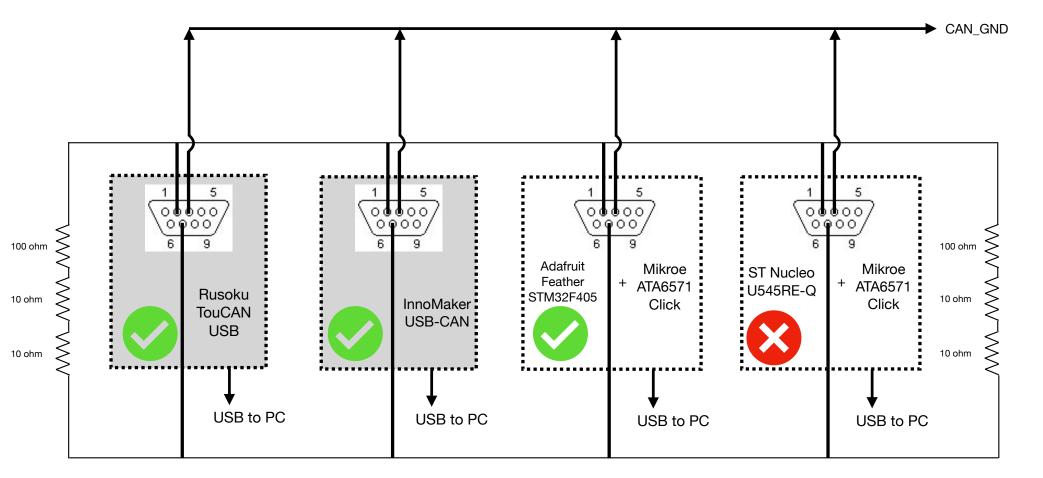
Basic CAN Network + GND Rusoku is running "can\_moni" CAN bus monitoring program. Successfully receives packets from InnoMaker and Adafruit STM32F405, but not from Nucleo U545RE-Q
