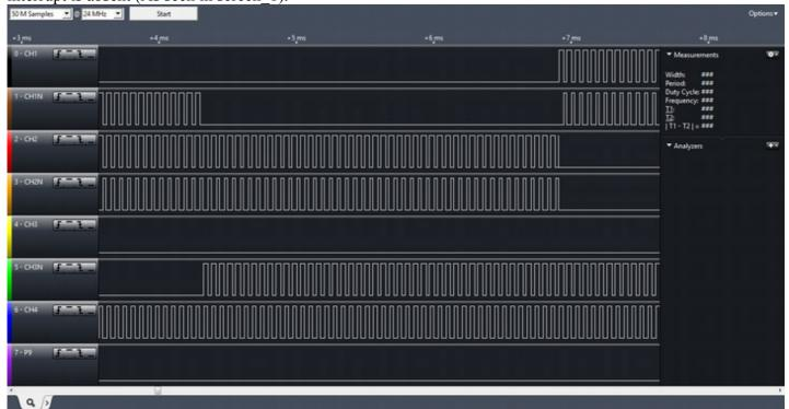
I plan to trigger ADC in Tim4 CH4 ISR. the code malfunction when I enable Tim4 CH4 interrupt (as seen in screen\_2 below). The CH1..CH3 and it complimentary output trigger spuriously.it also stop Timer3 counter from incrementing. It took me time to figure it out. The bad news is my code can't do with it. I don't know how to overcome the problem. I will appreciate all help I can get.
