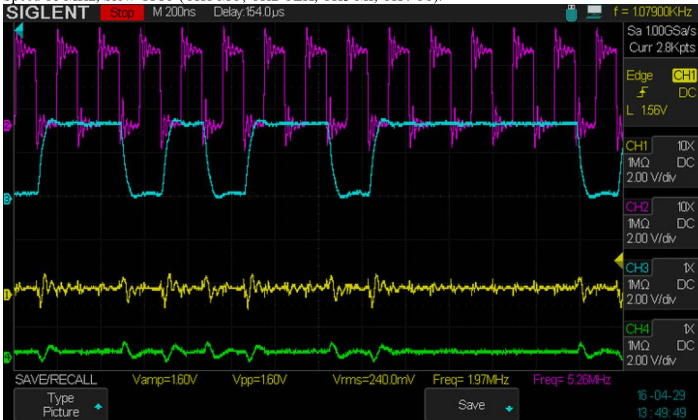
Speed 5 MHz, Fastest GPIO (CH1 MO, CH2 CLK, CH3 MI, CH4 CS).
