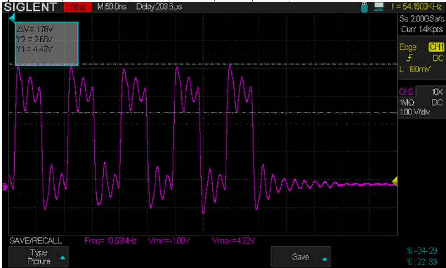
Speed 10 MHz, Medium GPIO + Pull Down enabled (CH1 MO, CH2 CLK, CH3 MI, CH4 CS).
