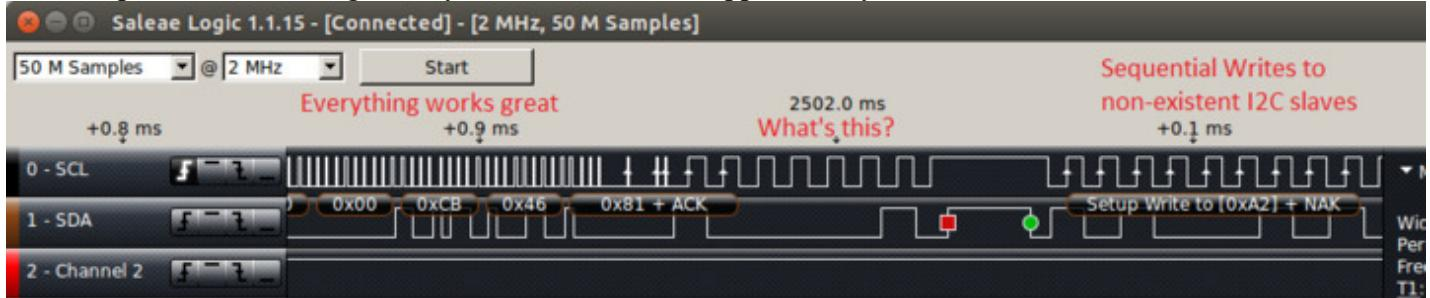
This picture shows the I2C bus correctly reading sequential data from an EEPROM. At some point, the STM32 acks a received byte and then the clock duty cycle changes for a bit. After that, it looks like the STM32 tries to cycle through various slave addresses (starting from the address of my EEPROM+2).
