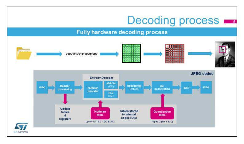
The decoding process follows the JPEG baseline algorithm: The file data are sent to the input FIFO. The file header is parsed and the corresponding internal RAM tables are updated. Once the header has been parsed, an interrupt can be raised. The compressed data are sent through the entropy decoder to generate the 8 by 8 Minimum Coded Units (MCUs) using the zigzag ordering. The resulting 8x8 tables are de-quantified and transformed through an inverse DCT (iDCT) into the original picture data.
