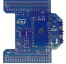
Environmental & Motion sensors (LSM6DS0 accelerometer & gyroscope, LIS3MDL magnetometer, LPS25H pressure, HTS221 humidity & temperature)
