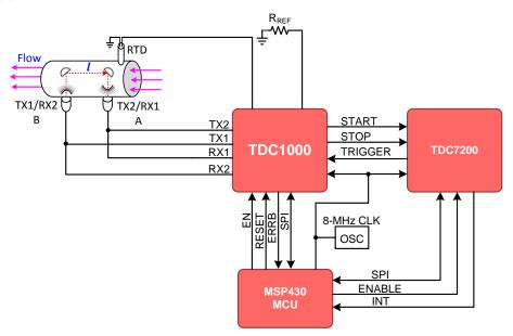
Figure 45. System in Time of Flight Mode
