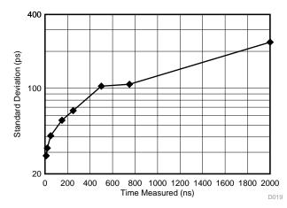
Figure 17. Measurement Mode 1 Standard Deviation vs. Measured Time-of-Flight
