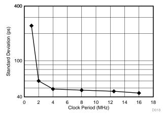
Figure 15. Standard Deviation vs. CLOCK
