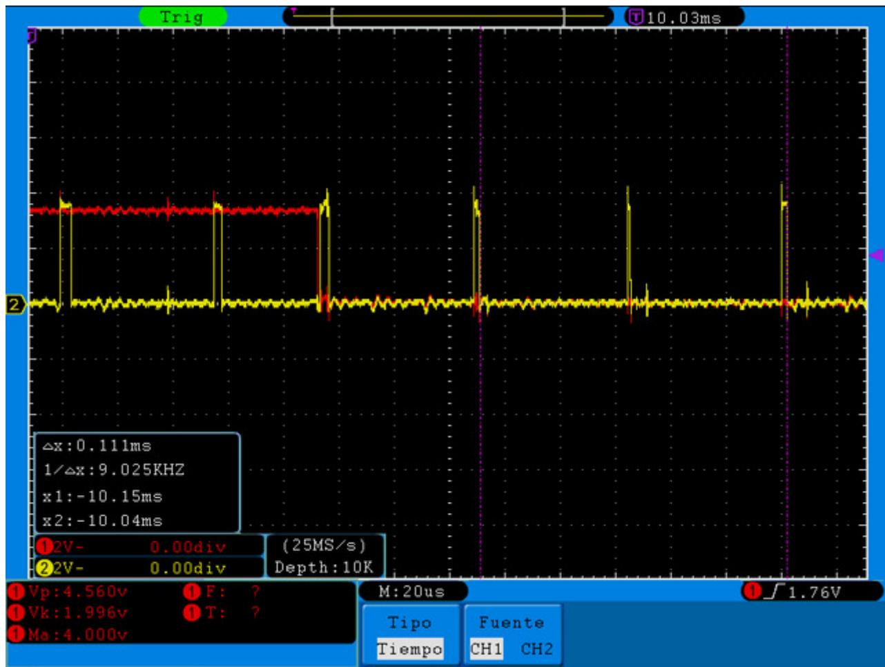
The modulation starts correctly on the third pulse, and when there is this displacement the modulation does not end correctly. This is the code:
