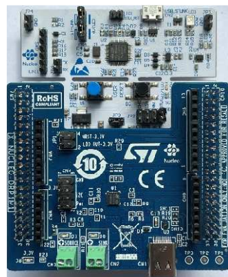
Figure 4 STM32 Nucleo 64 with X-NUCLEO-DRP1M1
