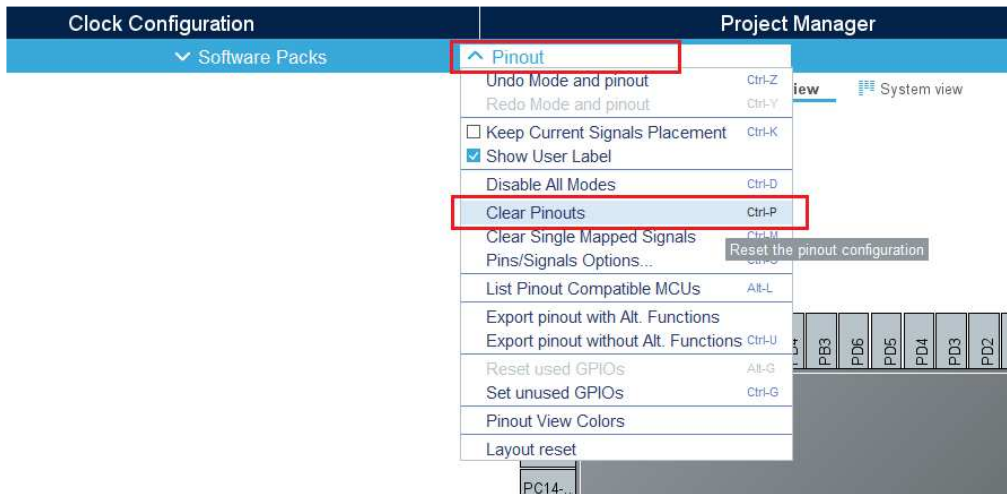
Figure 59 Clear pre-defined pinout
