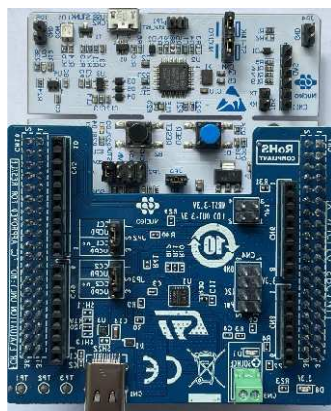
Figure 3 STM32 Nucleo 64 with X-NUCLEO-SRC1M1
