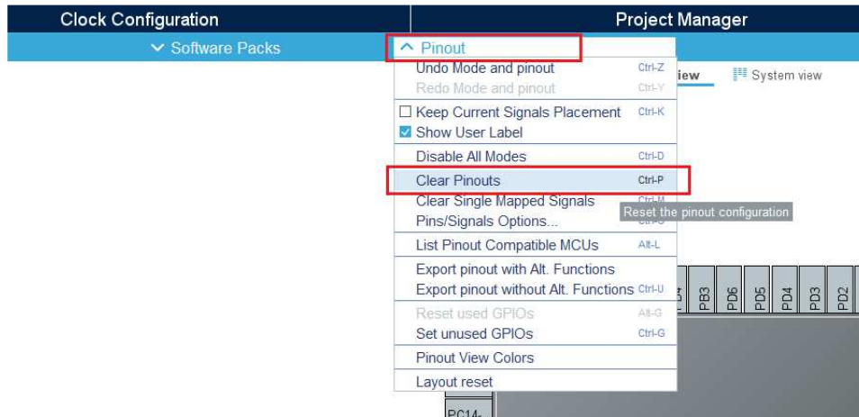
Figure 125 Source NoPD – Clear pre-defined pinout
