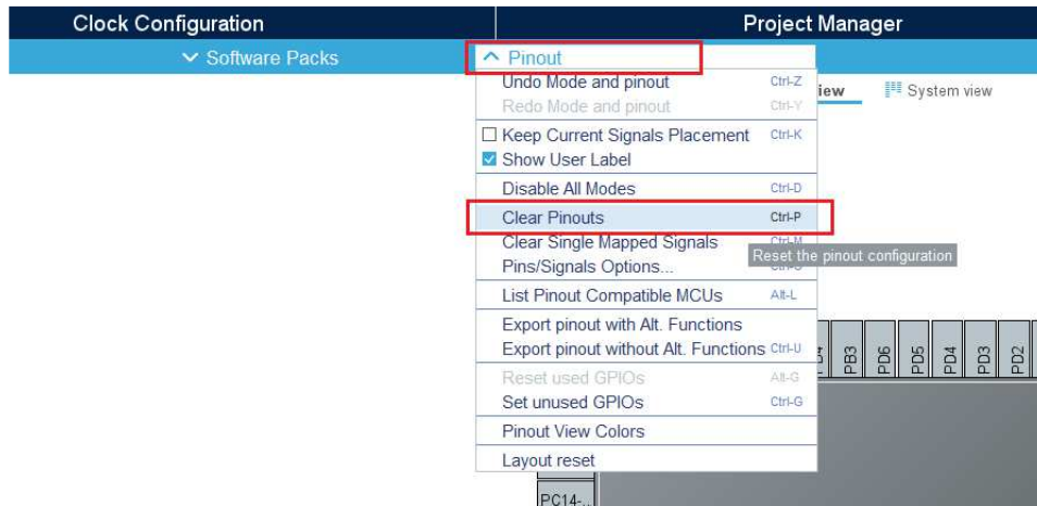
Figure 119 Source NoPD SRC1M1 – Clear pre-defined pinout
