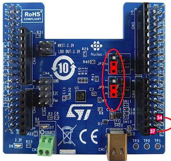
Figure 139 Source noPD – X-NUCLEO-SRC1M1 configuration
