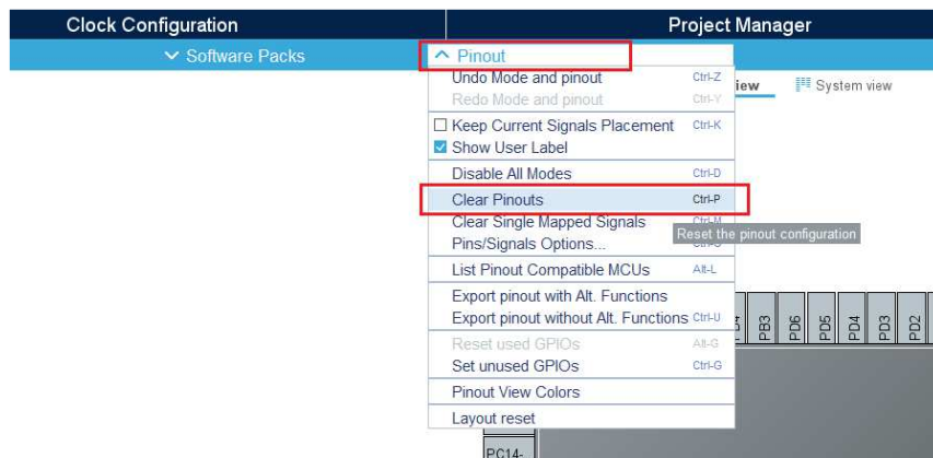
Figure 15 Clear pre-defined pinout
