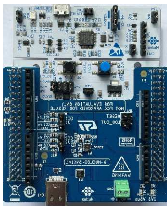
Figure 2 STM32 Nucleo 64 with X-NUCLEO-SNK1M1
