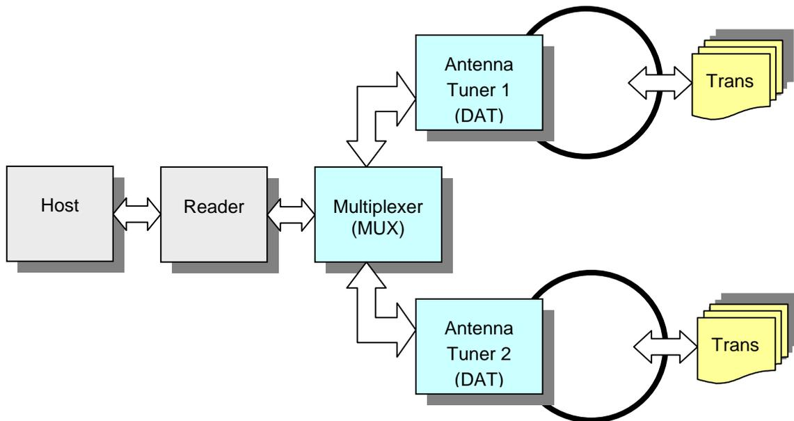
The picture above demonstrates also that external function units are arranged in hierachical order. The function unit class pattern this topology with a list of successors of type **FEDM\_ISCFunctionUnit**. Beginning with the first function unit after the reader one can traverse through the tree of function units.
