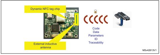
The design of an antenna for dynamic NFC tag is based on the placement of a loop on the application PCB. Its impedance matches the device internal tuning capacitance value  $(C_{tuning})$  to create a circuit resonating at 13.56 MHz. The basic equation of the tuning frequency is:
