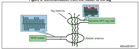
Figure 5. Communication from the reader to the tag
