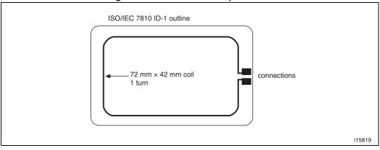
Figure 21. ISO standard loop antenna
