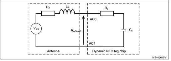
*Figure 8* shows the equivalent circuit of an dynamic NFC tag chip mounted on a loop antenna in the presence of a sinusoidal magnetic field.  $V_{OC}$  represents the open circuit voltage delivered by the antenna, which depends on the magnetic field strength, the antenna size and the number of turns.
