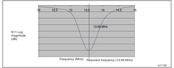
Figure 20. Example of the resonant frequency response of a prototype antenna
