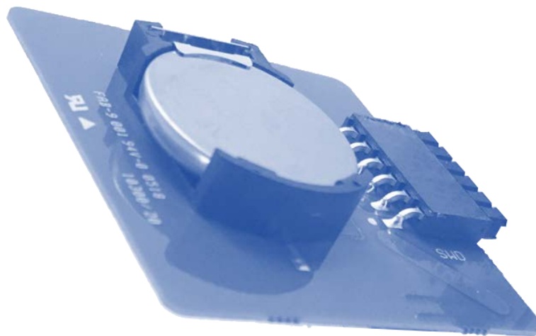
Figure 7. Battery inserted in cradle on rear of STEVAL-SMARTAG1 evaluation board
