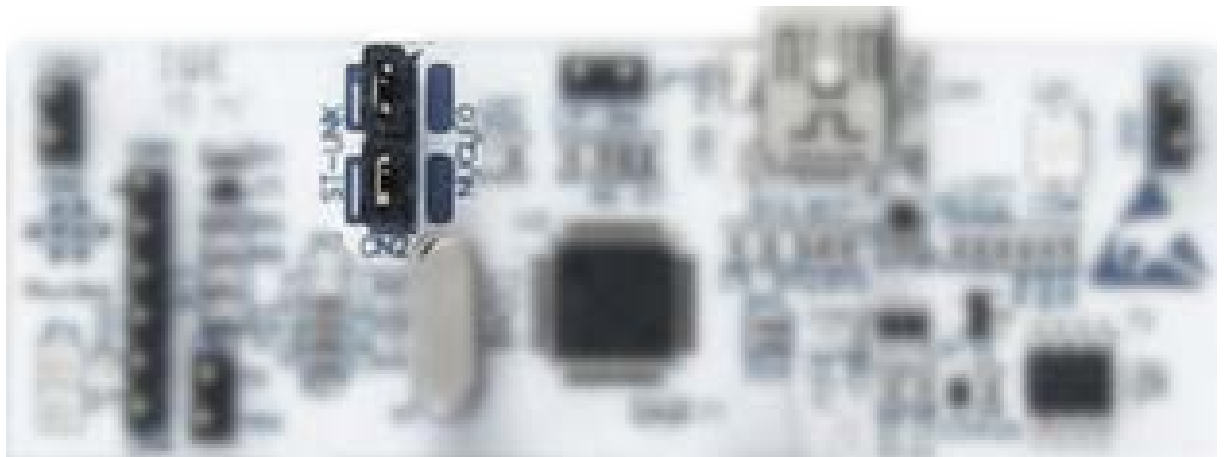
Figure 8. CN2 connector on ST-Link/V2 in-circuit debugger and programmer
