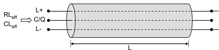
848 Figure 25 – Reference schematic for effective line capacitance and loop resistance
