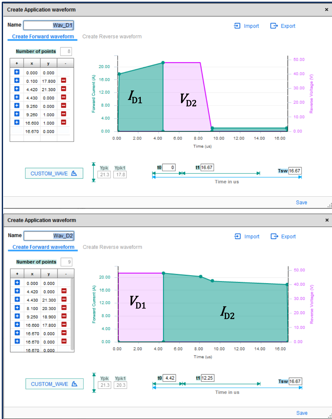
Figure 37: Reproduction of the forward waveforms
