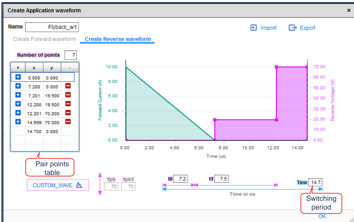
Figure 33: Entering flyback reverse voltage waveform
