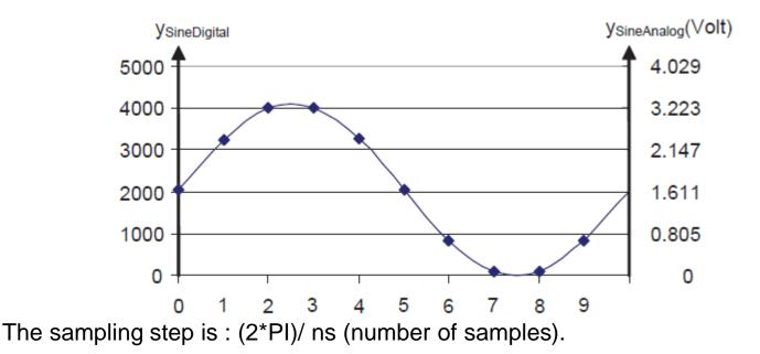
Because the result value of sin(x) is between -1 and 1, we have to recalibrate it to have a positive sinewave with samples varying between 0 and 0xFFF (which correspond, the range from 0 V to 3.3 V).
