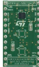
DIL24 Adapter ASM330LHH AIS2DW12* IIS2DLPC IIS2MDC ISM303DAC ISM330DLC LIS2DH12 LIS2DW12 LIS2MDL LIS3MDL* LPS22HH LPS33HW LSM6DSO LSM6DSOX LSM6DSR* STTS22H*
