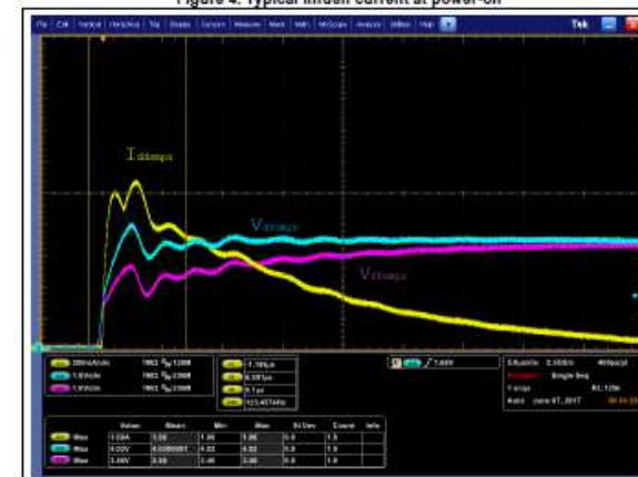
Figure 4. Typical inrush current at power-on
