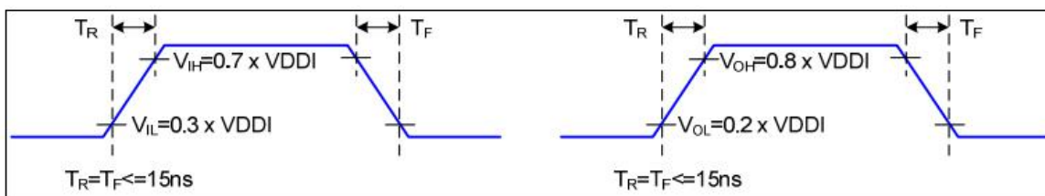
Figure 2 Rising and Falling Timing for I/O Signal
