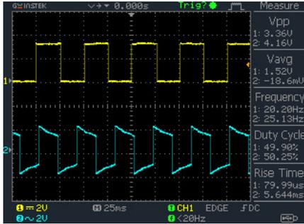
I had placed a toggle pin at VsyncEventCallback and FrameEventCallback to detect their rates. Yellow one represents Frame(field)rate while the blue one represents VSYNC frequency.
