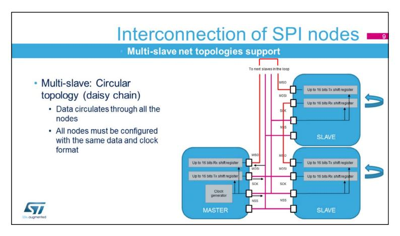
Another multi-slave configuration is the circular topology where all the data inputs and outputs of the nodes are connected together in a closed serial chain.
