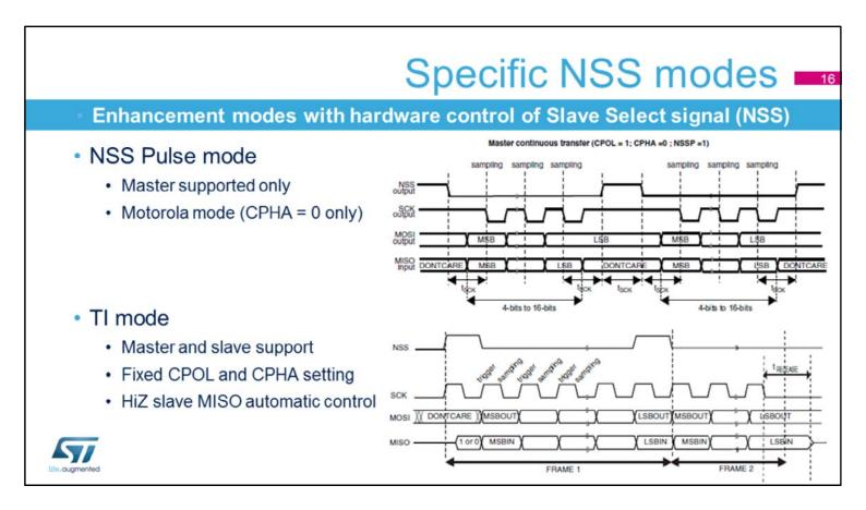
There are a few enhanced modes when the Slave Select signal is under specific hardware control.
