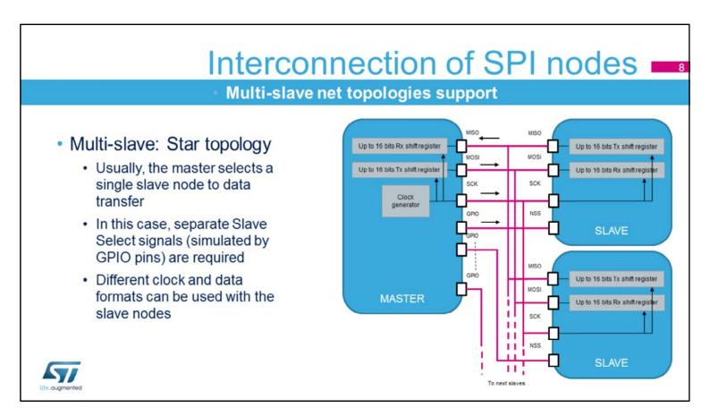
When the SPI network includes more than one slave, a star topology is commonly used when all the SCK, MOSI and MISO signals are interconnected.
