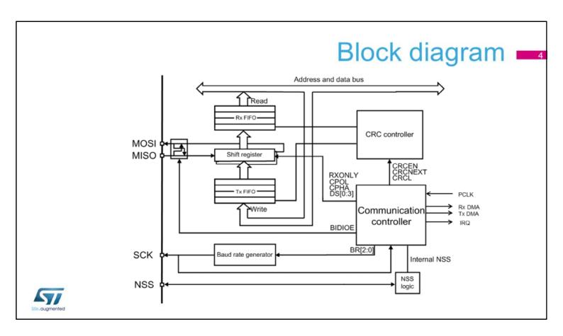
The simplified SPI block diagram shows its basic control mechanisms and functions. There are four I/O signals associated with the SPI peripheral. All of the data passes through receive and transmit buffers via their specific interfaces. The control block features are enabled or disabled depending on the configuration.
