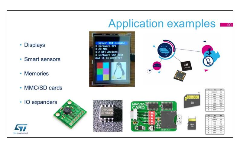
The SPI can be used in a wide range of applications where a simple data transfer is required without the need for a complex communication protocol. Secured transfers are also supported when used with smartcards.
