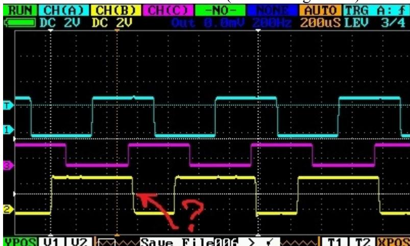
Yellow line is PC11. I've tried to change interface timer to TIM3/4 - no matter. Changing optimization level changes more than one waveforms. Init OC/IC changes more than one waveform. This is a complete
