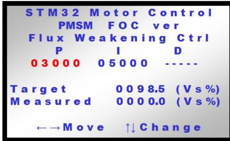
Figure 124: LCD screen for setting the P term of the flux-weakening PI
