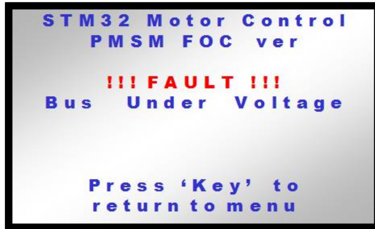
Figure 128: Error message shown in the event of an undervoltage fault
