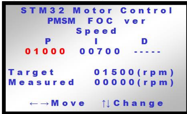
Figure 123: LCD screen for setting the P term of the speed PID
