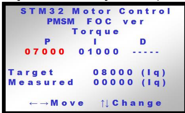
Figure 121: LCD screen for setting the P term of torque PID
