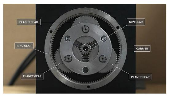
Sun gear teeth (Zs) = 21 Ring gear teeth (Zr) = 93 Gear ratio = Zs/Zr = 93/21 = 4.43
