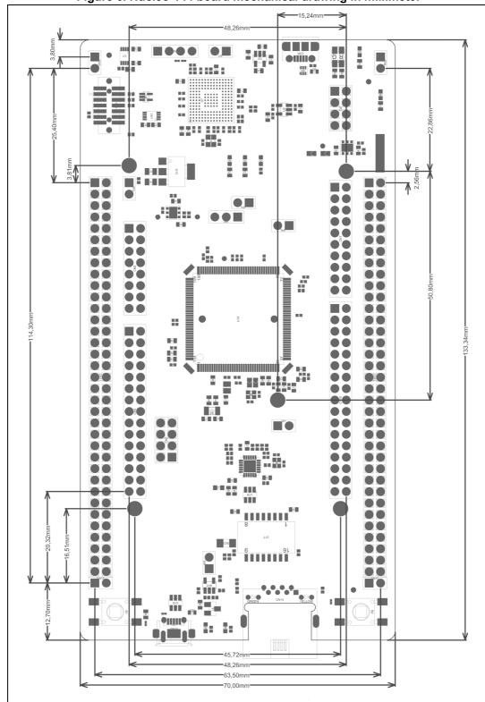
Figure 6. Nucleo-144 board mechanical drawing in millimeter
