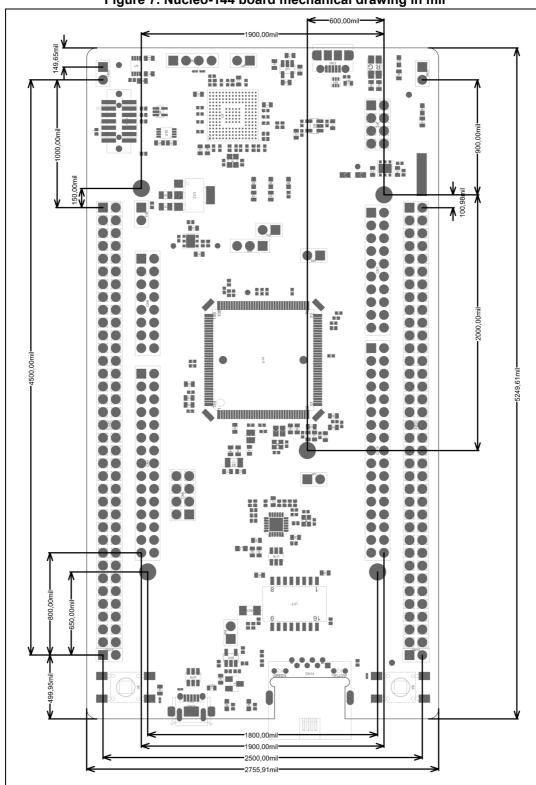
Figure 7. Nucleo-144 board mechanical drawing in mil
