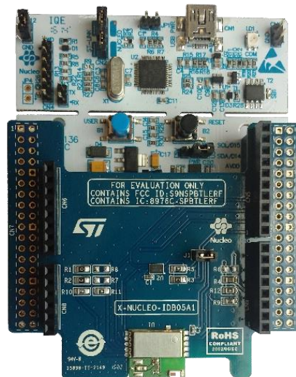
Figure 5 STM32 Nucleo 64 pins and X-NUCLEO-IDB05A1
