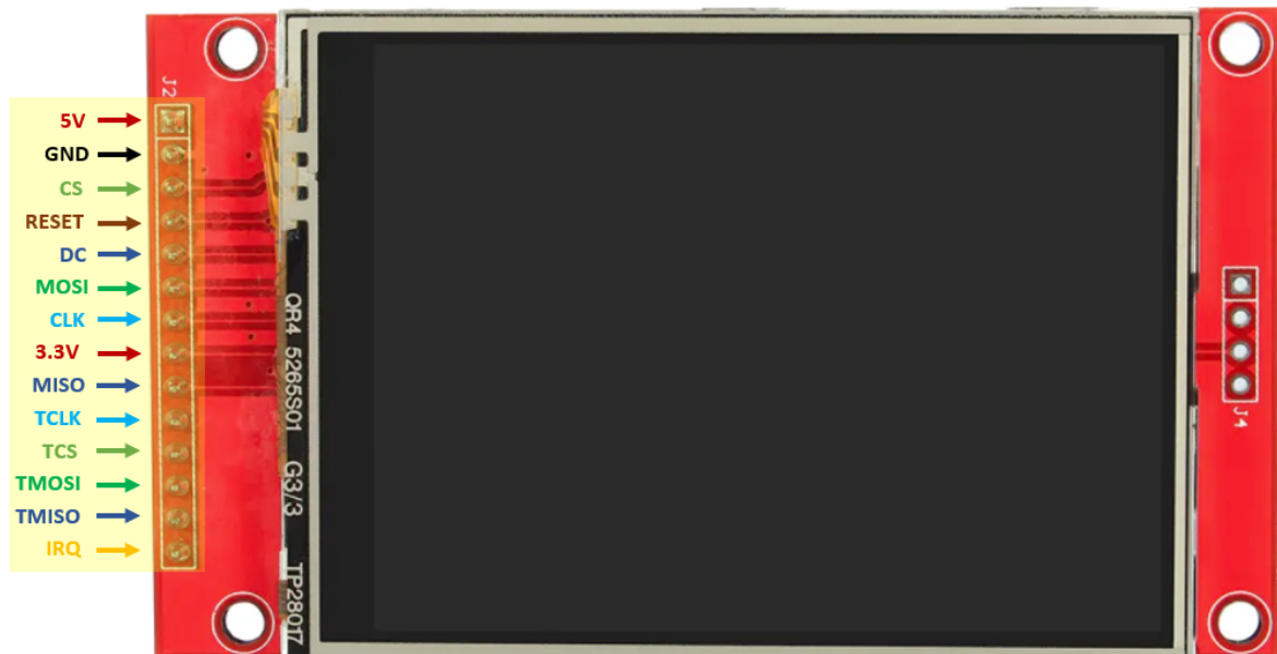
Figure 4.14: Infotainment GUI board connections
