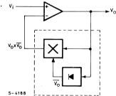
A compressor can easily be implemented with an expandor in the feedback path of an operational amplifier (Fig. 9). Assuming infinite gain for the amplifier:
