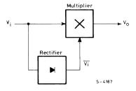
The output voltage  $V_o$  is proportional to the product of  $V_i$  and  $\overline{V_i}$ :
