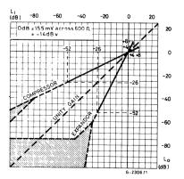
Fig. 4 - Comparison between LS150 performance (curve A) and limits from CCITT recommendation (curve B) - Green Book -Geneva 1972 - G162.
